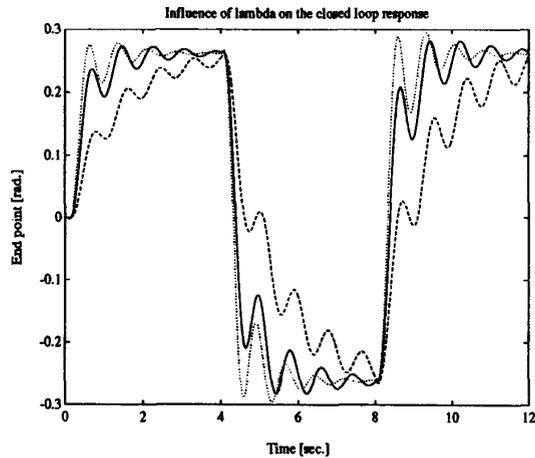
Figure 3: Effect of varying  $\lambda = 0.0008, 0.002, 0.008$  for fixed  $N_u = 6, N_2 = 30$ . The output response becomes slower and poles move towards the Laplace origin as  $\lambda$  is increased.
