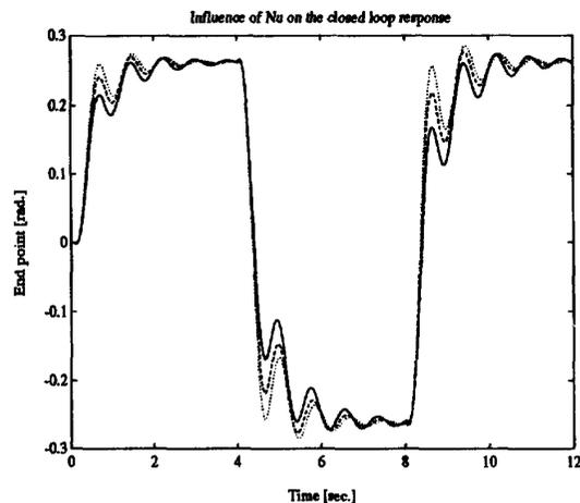
Figure 1: Effect of varying  $N_u = 2, 6, 10$  for fixed  $N_2 = 30$ ,  $\lambda = 0.002$ . The output response becomes faster and the poles move away from the Laplace imaginary axis as  $N_u$  increases.
