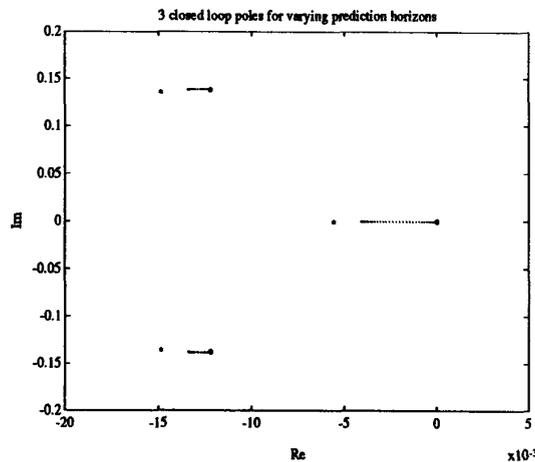
Figure 4: The closed-loop poles (omitting those of  $C_\delta(\delta)$ ) for  $\lambda = 0.1$  when  $N_2$  and  $1 + N_u$  grow from 1 (indicated by zeros) to 50.
