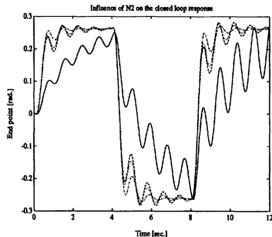
Figure 2: Effect of varying  $N_2 = 10, 20, 30, 40$  for fixed  $N_u = 6$ ,  $\lambda = 0.002$ . The output response becomes faster when  $N_2$  is increased.
