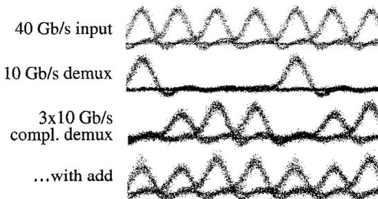
**ThN2 Fig. 2.** Measured BER vs. received power at 10 Gbit/s for simultaneous add and drop. Drop sensitivity =  $-34.4$  dBm; Total system penalty for clear/add (including EAM demux) =  $2.4$  dB =  $>$  Add penalty =  $\sim 1.3$  dB. Eye diagrams show original 40 Gb/s signal, simultaneous SOA-MZI demux and complementary demux without and with add.
