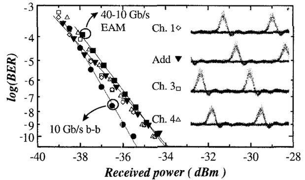
**ThN2 Fig. 3.** Measured BER vs. received power at 10 Gbit/s for all channels at optimised add operation. Add penalty  $< 0.3$  dB relative, subtracting EAM demux penalty. Eye diagrams shown for all channels after EAM demux.
