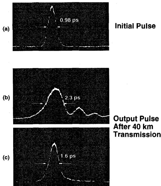
**ThN1 Fig. 3.** Measured optical pulse waveforms: (a) Initial pulse; (b) After 40-km transmission with dispersion slope of 0.06 ps/nm<sup>2</sup>/km; (c) After 40-km transmission with dispersion slope of 0.02 ps/nm<sup>2</sup>/km.
