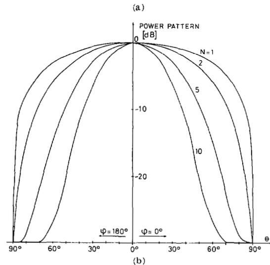
Fig. 2. (a) Power pattern for one MSA. \$P(\theta) = 1 + \cos^N \theta\$. Dashed curve shows pattern of crossed-dipole in plane bisecting arms. (b) Power pattern for one MSA. \$P(\theta) = 1 + 1000 \cos^N \theta\$.
