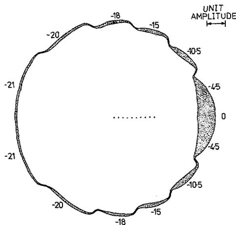
Fig. 5. Near-field amplitude distribution from Hansen-Woodyard array.
