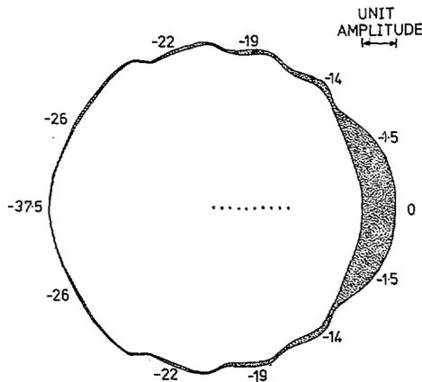
Fig. 4. Near-field amplitude distribution around ordinary endfire array.
