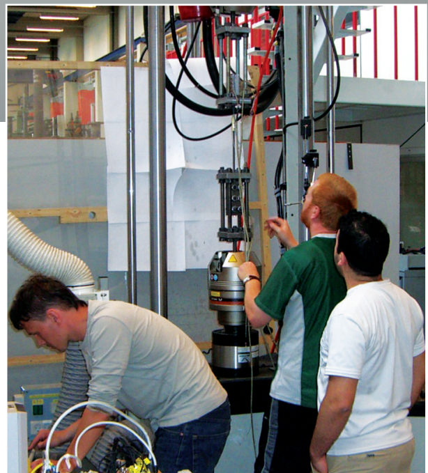
Testing the new anchor as part of a Master's project at DTU Civil Engineering. Photo: Jacob W. Schmidt
