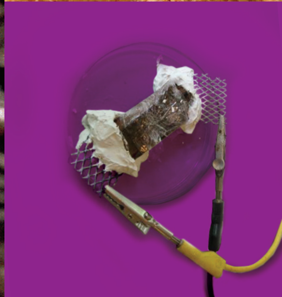
Removal of alum from archeological wood using an applied electric field. Experimental set-up
