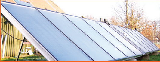
Solar collectors being tested at the Department of Civil Engineering. Photo: Jianhua Fan
