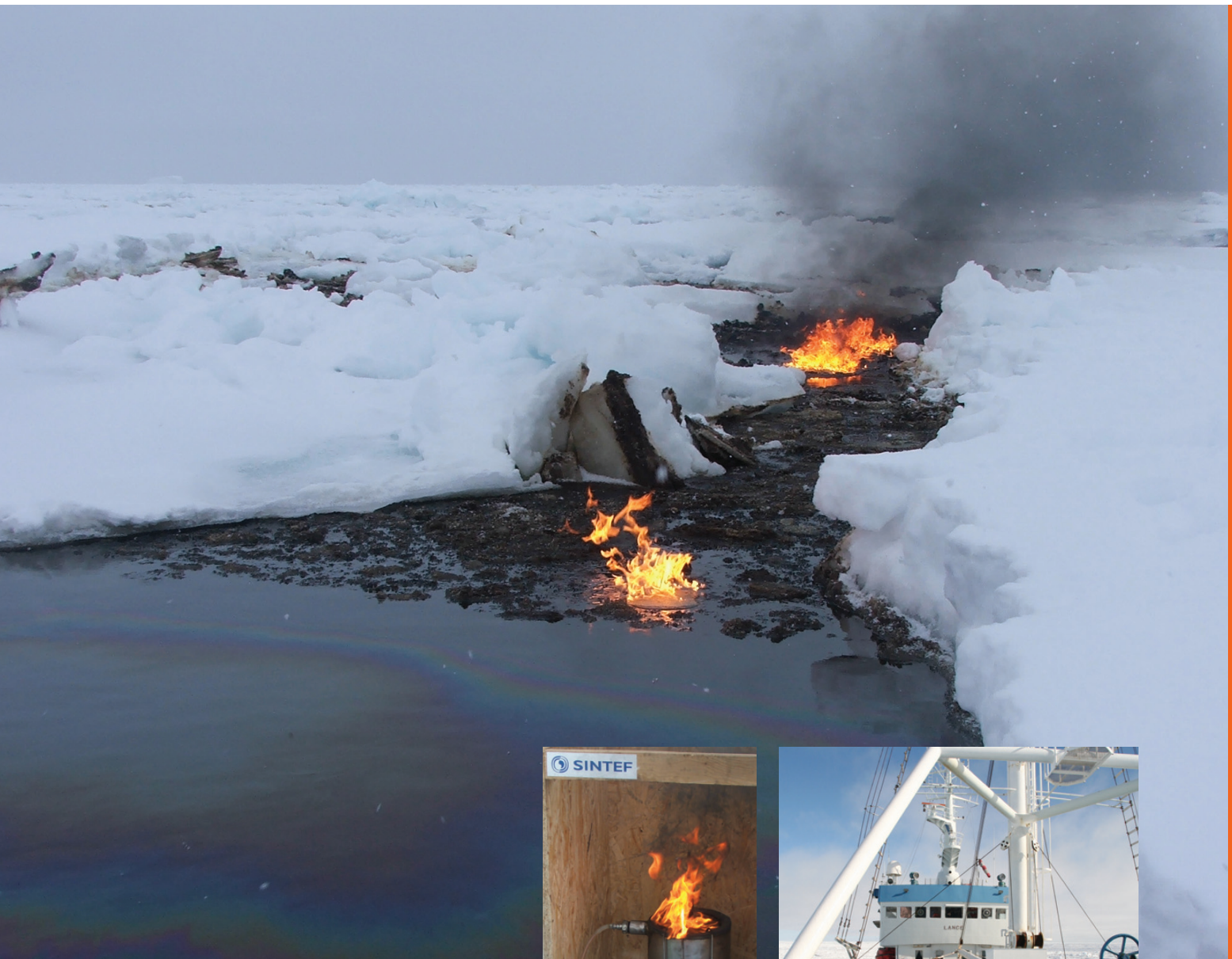
Burning of experimental oil spill in the Barents Sea and small-scale burning. Photo: Janne Fritt-Rasmussen
