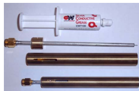
Fig. 16. Illustration of the sleeve balun and the conductive glue.
