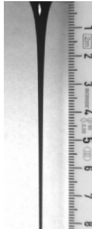
FIG. 3. General view of a viscous thread, 8 cm down from the outlet.
