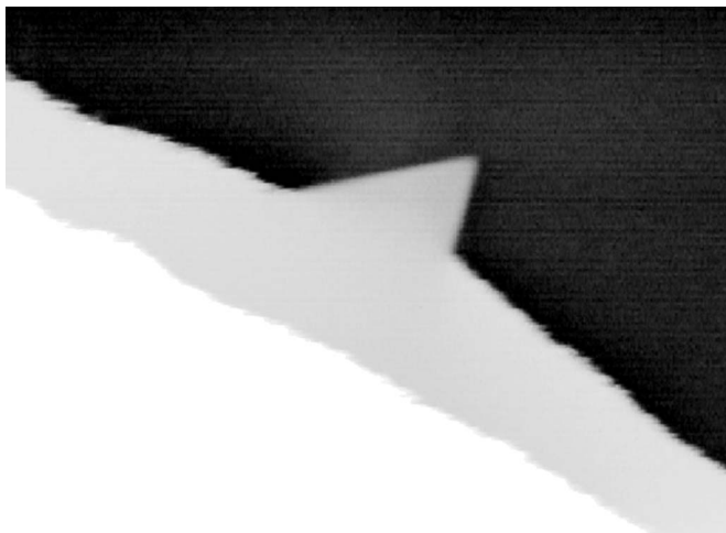
FIG. 5. Lomer-Cottrell lock pinning a step. Note that the step edges of the Lomer-Cottrell lock are not frizzy at all compared to the ordinary Au(111) steps ( 500 \text{ \AA} \times 365 \text{ \AA} ).
