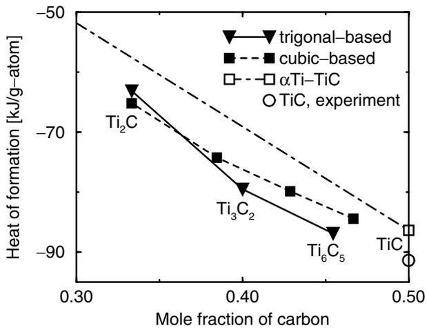
FIG. 4. The calculated heat of formation for vacancy-ordered structures in  $TiC_x$ . The experimental value for TiC is taken from Ref. [30].
