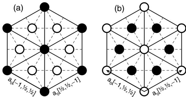
FIG. 3. Ordered structures within the partially filled  $(111)_{B1}$  carbon layers of  $Ti_3C_2$  (a) and  $Ti_6C_5$  (b). Carbon atoms are shown by full circles, vacancies by open circles.
