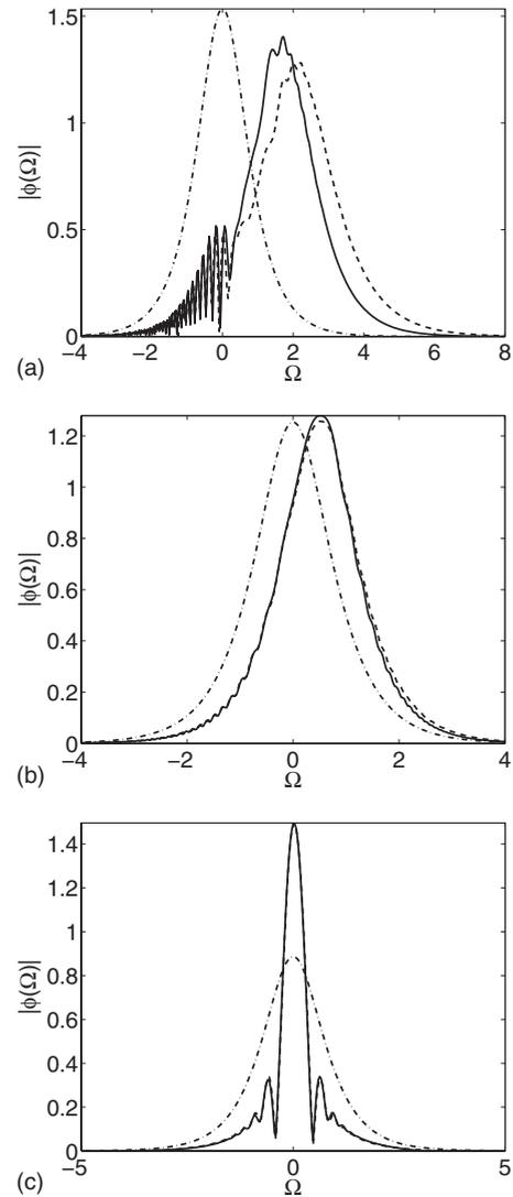
FIG. 9. Simulation pulse-spectrum at pulse energies (a)  $1.5E_s$ , (b)  $E_s$ , and (c)  $0.5E_s$  at rescaled distances of  $\zeta=0$  (dot-dashed line) and  $\zeta=25$  with (solid line) and without (dashed line) third-order dispersion.
