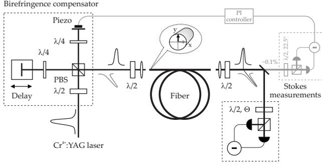
FIG. 3. Schematic of the single-pass method for the efficient production of polarization squeezed states. The Stokes measurement after the fiber scans the dark  $\hat{S}_1$ - $\hat{S}_2$  plane of the circularly  $\langle \hat{S}_3 \rangle \neq 0$  polarized output.
