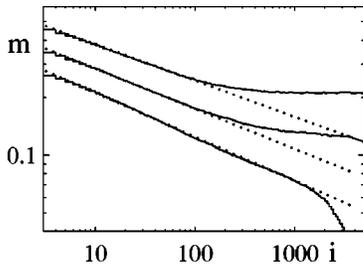
FIG. 15. Average activity  $m$  for  $c=0.1$ ,  $d=0.01$  in an ensemble of 20 systems of  $L=20\,000$ , showing the appearance of quasi-power-law decay. The three curves correspond to  $p=0.612$ ,  $0.616$ , and  $p=0.62$ , respectively, and are shifted by 30% for clarity. The three straight lines corresponds to power laws with exponents  $-0.19$ ,  $-0.21$ , and  $-0.23$ . In particular, the scaling in the system for  $p=0.612$  looks rather convincing with an exponent of  $-0.23$ .
