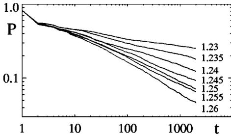
FIG. 9. Average survival probabilities for spreading clusters in our CML with  $r=3$  and  $b=0.2$  for various values of the background (indicated in the figure). The natural background state has  $u=1.235$ .
