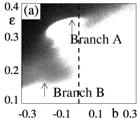
FIG. 2. Activity in the model, Eqs. (2) and (3), at  $t=1000$ . White regions correspond to points in the  $(\varepsilon, b)$  plane where the initial activity has decayed into an absorbing configuration and the darker regions to points with a nonvanishing order parameter. Clearly the transition curve becomes quite complicated; the two branches discussed in this paper are indicated as “Branch A” and “Branch B” (see text). The dashed line indicates the Chaté-Manneville model ( $b=0$ ).
