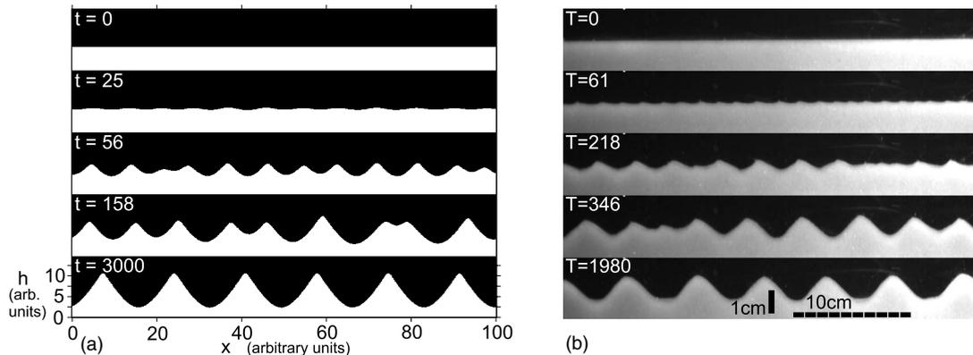
FIG. 2. Temporal development of flat bed instability. (a) For the amplitude equation (3),  $\epsilon = 0.03$  and  $\delta = 1$  with periodic boundary conditions. (b) In the experiment [side view of the central region (36 cm) of the channel]. The length of each black bar is 1 cm—note that the vertical scale is twice that of the horizontal.  $T$  denotes the number of oscillations.
