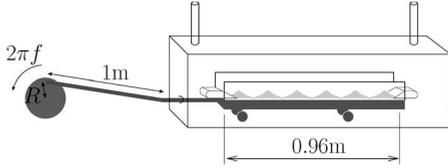
FIG. 1. The experimental setup: A narrow channel with a layer of sand is moved periodically in a plexiglass tank.
