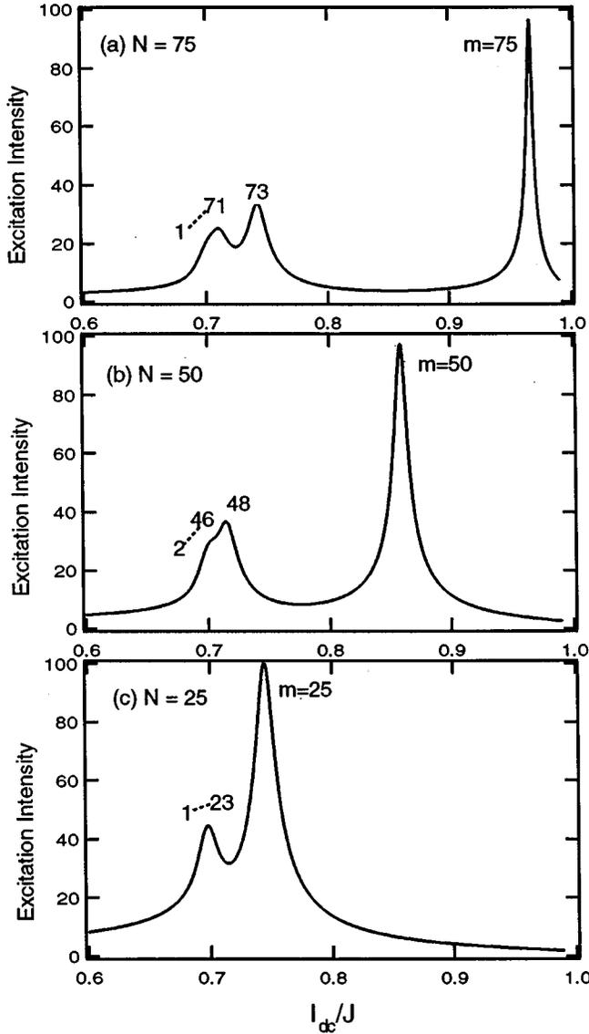
FIG. 3. Bias current dependence of the resonance intensity. For calculation,  $\omega/\omega_{p0}=0.85$ ,  $k\lambda_J=0.02$ ,  $\alpha=0.01$ , and  $1+2S=4.5 \times 10^{-6}$  were assumed. (a)  $N=75$ , (b)  $N=50$ , and (c)  $N=25$ . The peak position at the  $m=N$  mode strongly depends on the stacked junction number  $N$ . The lower number mode peaks are merged together, and its position is insensitive to  $N$ .
