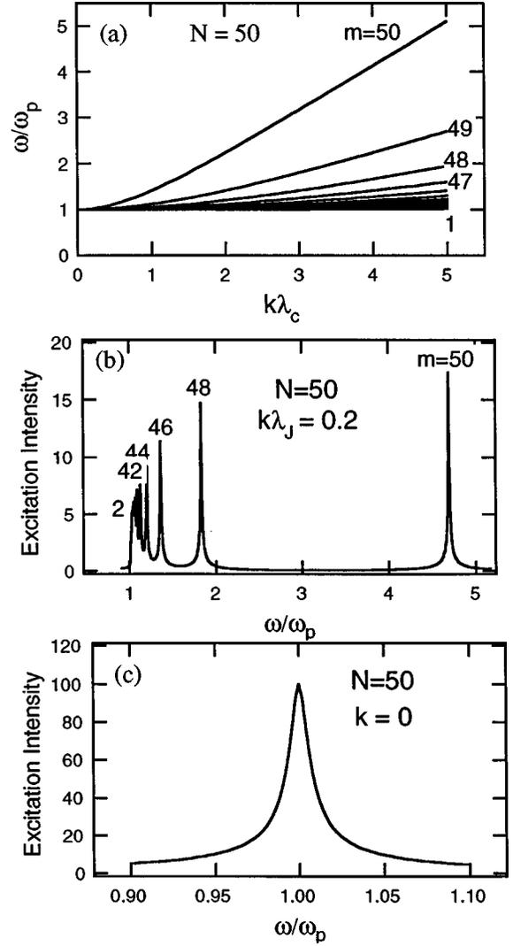
FIG. 2. (a) Plasma dispersion relation curves for  $N=50$ . Used parameters are  $d=1.2$  nm,  $t=0.3$  nm, and  $\lambda_L=200$  nm.  $\lambda_c$  is the scaling length of the all in-phase mode  $m=N$ . (b) and (c) Frequency dependence of the resonance intensities at (b)  $k=0.2 \cdot \sqrt{\cos \phi^{(0)}}/\lambda_J$  and (c)  $k=0$ .  $\alpha/\sqrt{\cos \phi^{(0)}}=0.01$  is assumed. The resonance intensity was evaluated by  $\sum_i |A_{ii-1}|/N$ .
