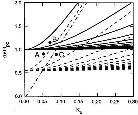
FIG. 5. Schematic graph showing relationship between the plasma dispersion curves and the  $k$ - $\omega$  conditions. A set of solid curves is the dispersion of possible eigenmodes at  $B_{dc}=0$ , and a set of dashed curves is the dispersion when  $B_{dc}$  is some nonzero value. The all in-phase mode dispersion approaches asymptotically to the dash-dot line in the figure with much increasing  $\omega/\omega_{po}$ , regardless of the  $B_{dc}$  magnitude.
