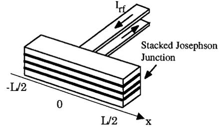
FIG. 4. Experimental configuration demonstrating that the bias current forms a standing wave. Since the Fourier components have forms of  $\cos(kx-\omega t)+\cos(kx+\omega t)$ , the analysis in the present paper can be used directly.
