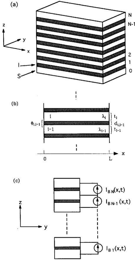
FIG. 1. (a) Schematic picture of a vertically  $N$ -stacked Josephson junction. (b) Enlarged diagram showing the parameter notation for convenience. (c) A stacked junction system with a bias current set.
