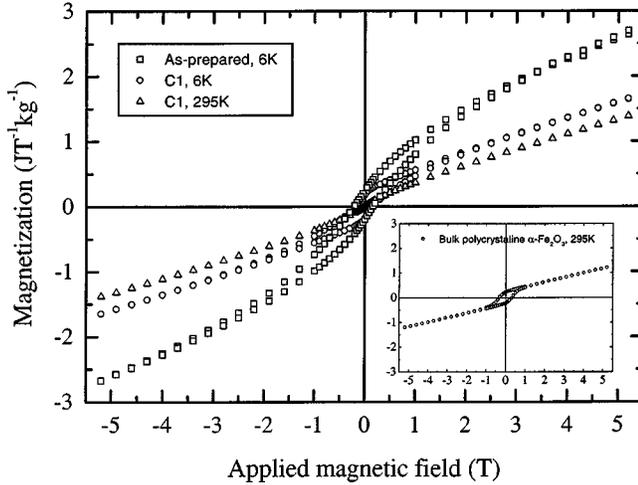
FIG. 9. Hysteresis loop of the as-prepared sample ( $\square$ ) and of the dried sample *C1* at 6 K ( $\circ$ ) and 295 K ( $\triangle$ ). The magnetization is given per unit mass of  $\text{Fe}_2\text{O}_3$  in the sample as determined by AAS. The inset shows the hysteresis loop of sample *B* measured at 295 K.
