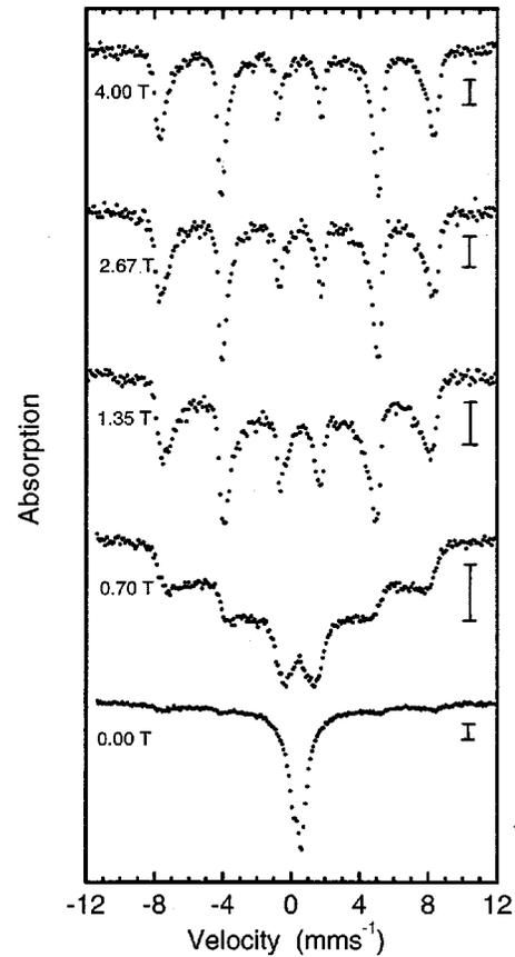
FIG. 5. Mössbauer spectra of sample *C1* obtained at 230 K in zero field and in different applied magnetic fields. The field of 0.7 T was applied perpendicular to the gamma-ray direction, while the larger fields were applied parallel to the gamma-ray direction. The vertical bars represent 1% absorption.
