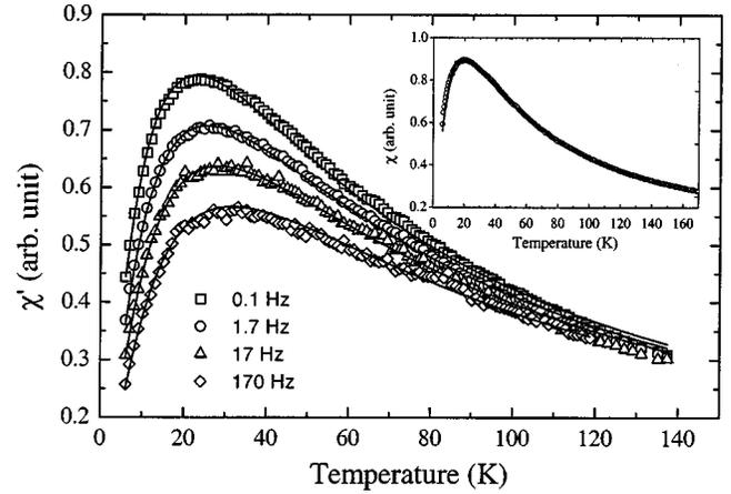
FIG. 10. The real part of the ac magnetization curves measured at the frequencies  $f = 0.1, 1.7, 17,$  and  $170$  Hz after cooling in zero field. The inset shows the ZFC magnetization curve measured with an applied field of 2.0 mT. The solid lines are fits to the data based on the models described in the text.
