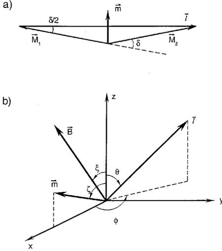
FIG. 1. (a) Illustration of the canting angle  $\delta$  between two sublattice magnetizations  $\mathbf{M}_1$  and  $\mathbf{M}_2$ , the resulting magnetization  $\mathbf{m} = \mathbf{M}_1 + \mathbf{M}_2$ , and the vector  $\mathbf{l} = \mathbf{M}_2 - \mathbf{M}_1$ . (b) Definition of angles in a spherical polar coordinate system with the  $z$  axis being the [111] orthorhombic direction.
