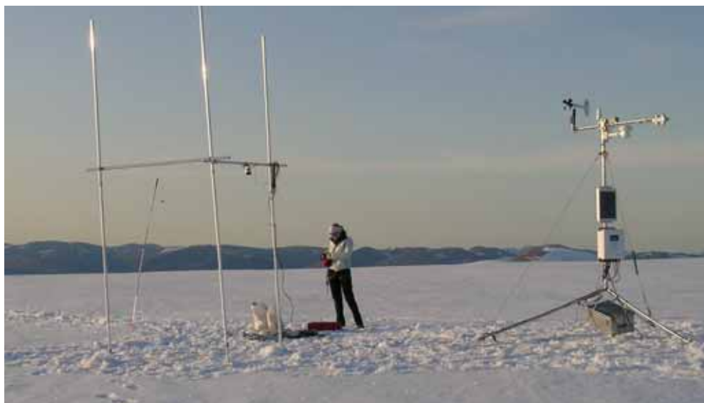
Figure 3.5 The AWS3 station near the summit (initial establishment 5 April 2008). The stakes supporting the sonic range sensors are ready to be raised next year. Being in the accumulation area, either the tripod will have to be dug out of the snow or the mast extended. Photo: Michele Citterio, GEUS, Copenhagen.
