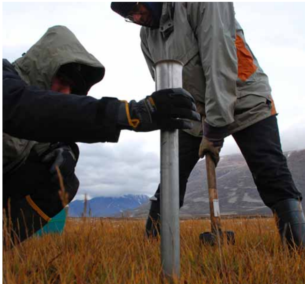
Figure 6.8 Hammering the steel pipe into the permafrost. Photo: Torbern Tagesson.
