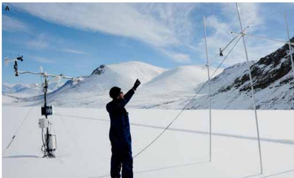
Figure 3.3 a) The tilted structures supporting the sonic ranger that was fixed 13 May 2009. b) The AWS1 station (initial establishment, 29 March 2008). Photo: Michele Citterio, GEUS, Copenhagen and Gernot Weyss.
