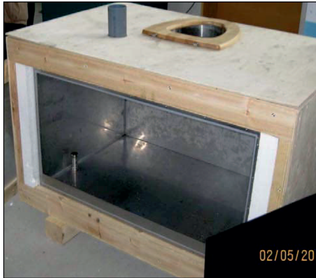
Figure 2.2. A demonstrating model of the composting toilet that will be tested in a selected tourist hut in Qeqqata municipality (Picture: Ragnhildur Gunnarsdóttir).
