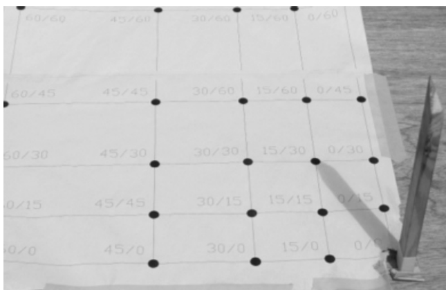
Fig. 3. Solar pointer and measurement grid, the current IA is azimuth of 15^\circ and altitude 30^\circ .
