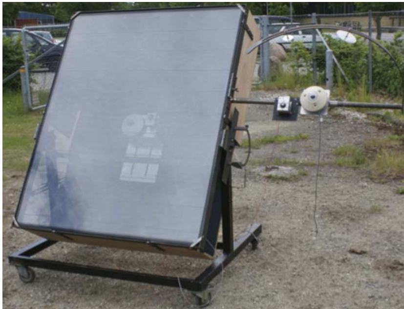
Figure 4.2: Movable measurement test rig with sample mounted.
