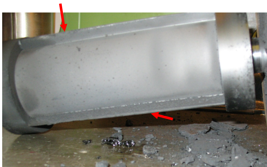
Figure 6.1. Image of inner wheel of pyrolysis centrifuge reactor
