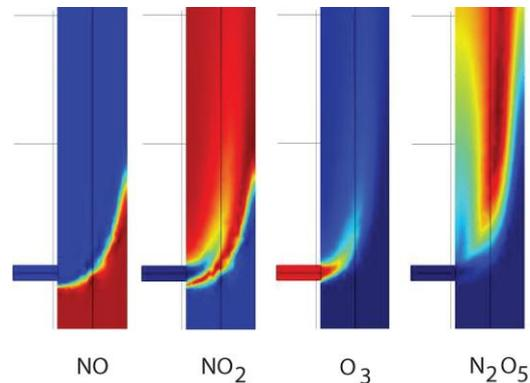
Fig. 3 Concentrations of NO, NO<sub>2</sub>, O<sub>3</sub> and N<sub>2</sub>O<sub>5</sub> for J=4, corresponding to A-B region in Fig. 2.
