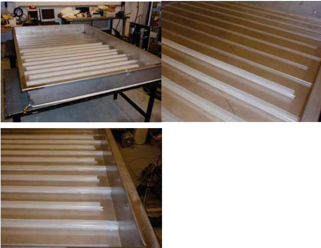
Fig. 4: Photos of the heat storage module with silicone pipes attached to the upper surface.
