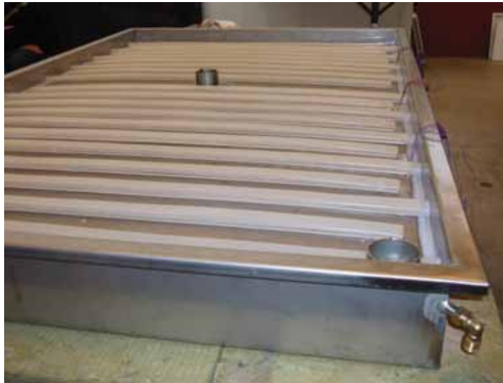
Fig. 1: Photo of the PCM heat storage test module with plate heat exchangers at the top and the bottom.
