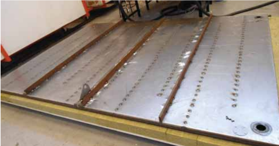
Figure 8: Photos of the second heat storage module with two holes used to fill in the salt water mixture.
