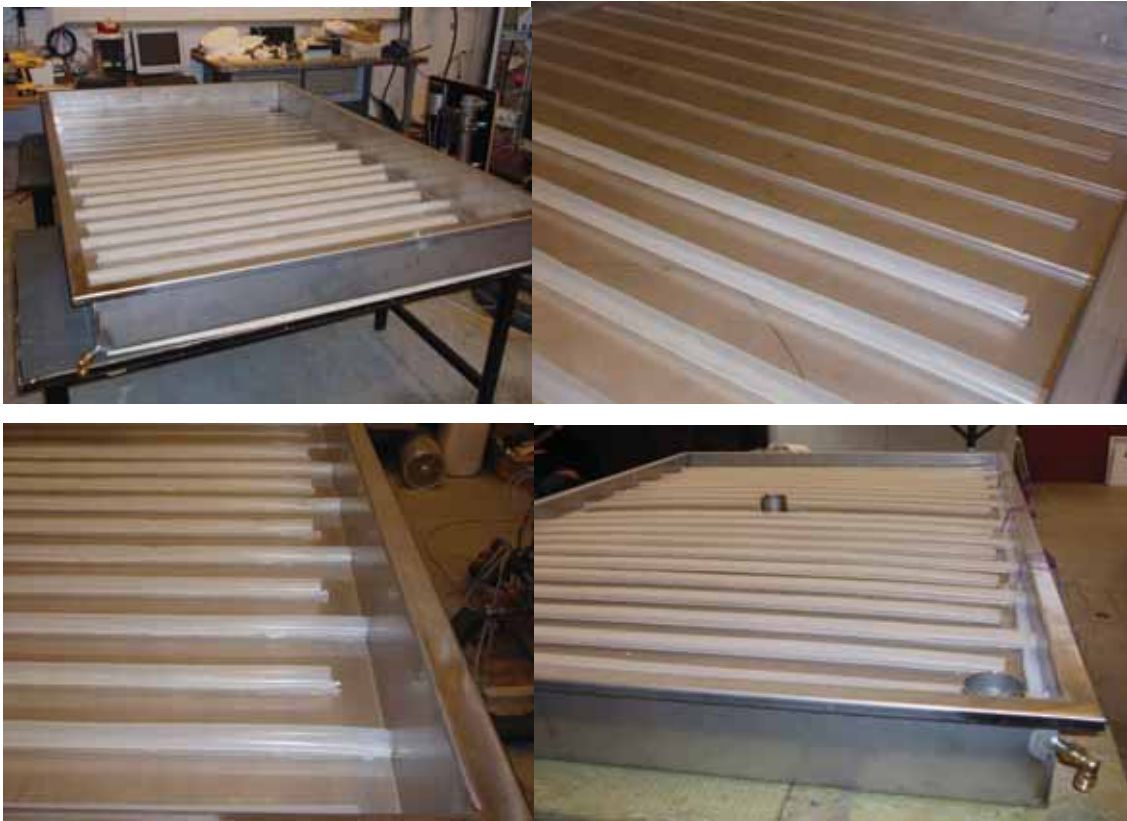
Fig. 4. Photos of the first heat storage module with silicone pipes attached to the upper surface.
