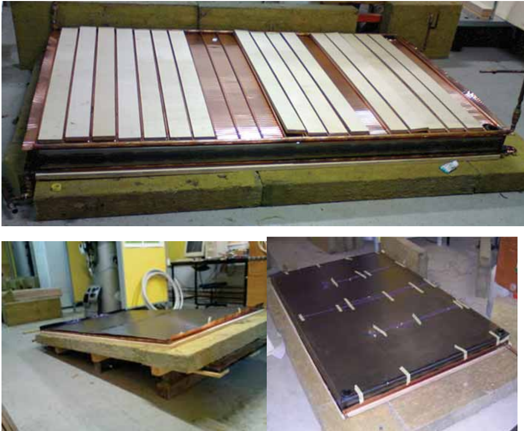
Figure 5: Photos of the first heat storage module.
