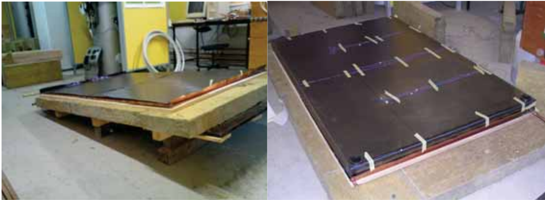
Fig. 3: Photos of the heat storage module with a copper absorber used for the heat transfer.
