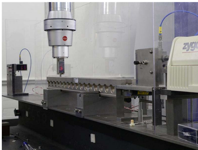
Fig 1. Measurement of a step gauge using the Step Gauge Rig mounted on the Leitz CMM
