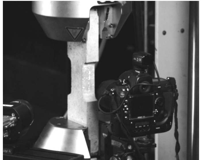
Figure 4: reinforced prism in tensile test setup.
