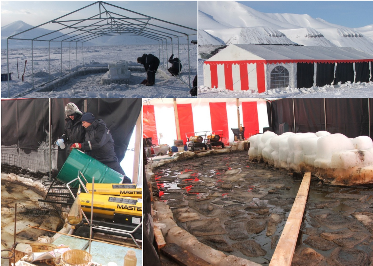
Figure 3.2.4 Preparation of the weathering flume in the fjord ice (upper left). Tent placed over the flume to control air temperature (upper right). Oil applied to the flume (bottom left). 90 % ice cover weathering experiment (bottom right).
