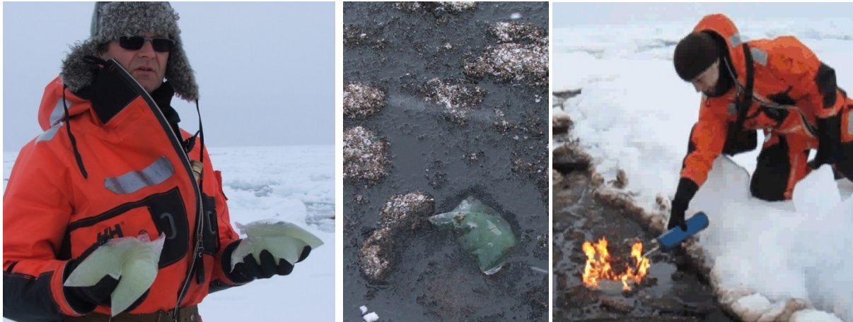
Figure 3.3.2 Gelled gasoline in plastic bags ready for use, placed in the oil slick and ignited right (right photo: Per Johan Brandvik).
