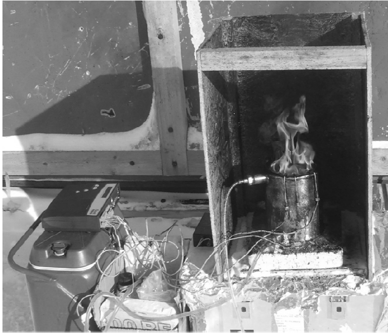
Figure 1 Burning cell unit in the field, thermos to warm cooling water and temperature logger to the left.
