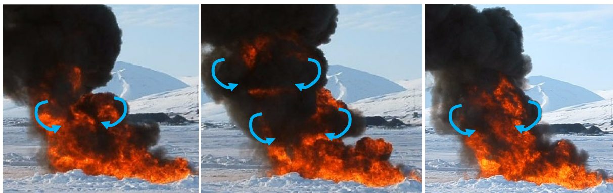
Figure 2.1.2 Oscillation of the flames during burning Troll B crude oil in a basin cut in the fjord on Svalbard 2008. Snap shots from video filming of the burning.
