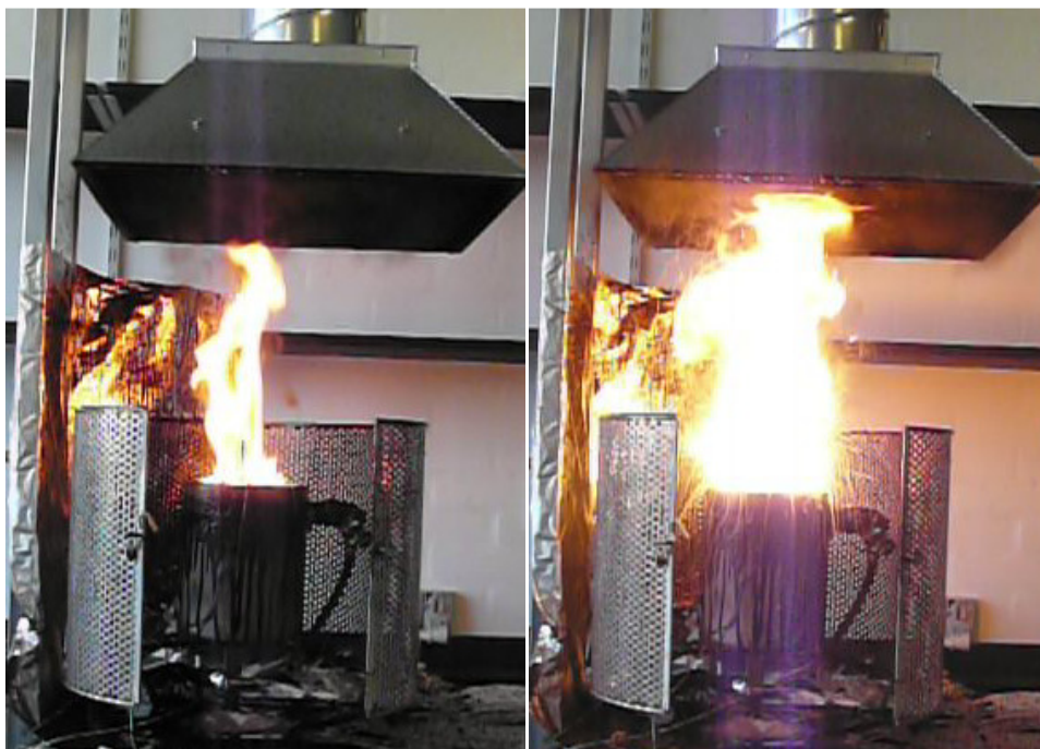
Figure 2.1.3 Burning of a fresh Troll B crude oil sample 2 minutes after ignition (left) and the vigorous phase at the end of the burning just before flame out (right).
