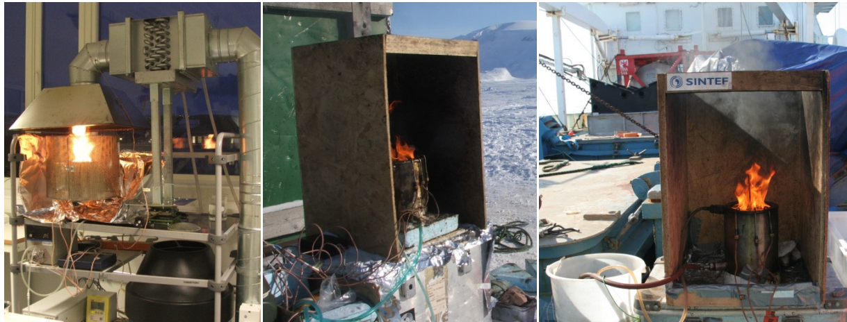
Figure 4.3.1 Use of the burning cell in different situations. The burning cell used in the laboratory with the exhaust system and protection shield (left). The burning cell on the fjord ice at Svea, Svalbard (middle) and on deck of the research vessel in the Barents Sea (right). The wind shield and how the hoses for the cooling system were warmed can also be seen.
