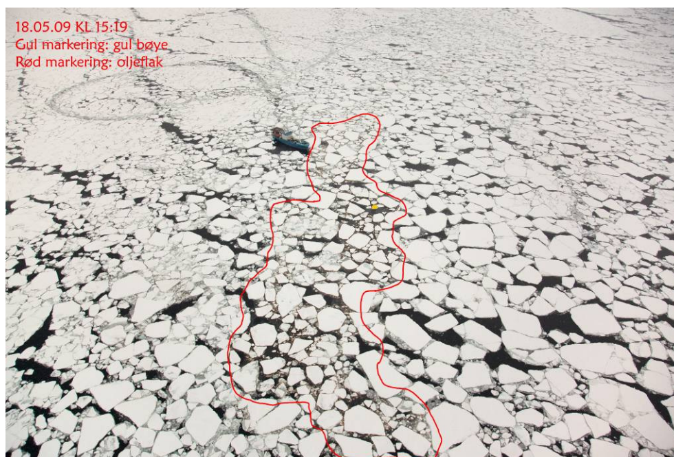
Figure 1 The spreading of the 7 m 3 oil spill in ice three days after the oil release (Barents Sea, May 18 th , 2009).
