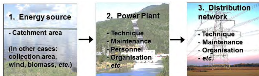
Figure 11.5. The functional model provides an overview of those functions of the examined power plant which are to be taken into account in the risk analysis process (Molarius et al. , 2010).
