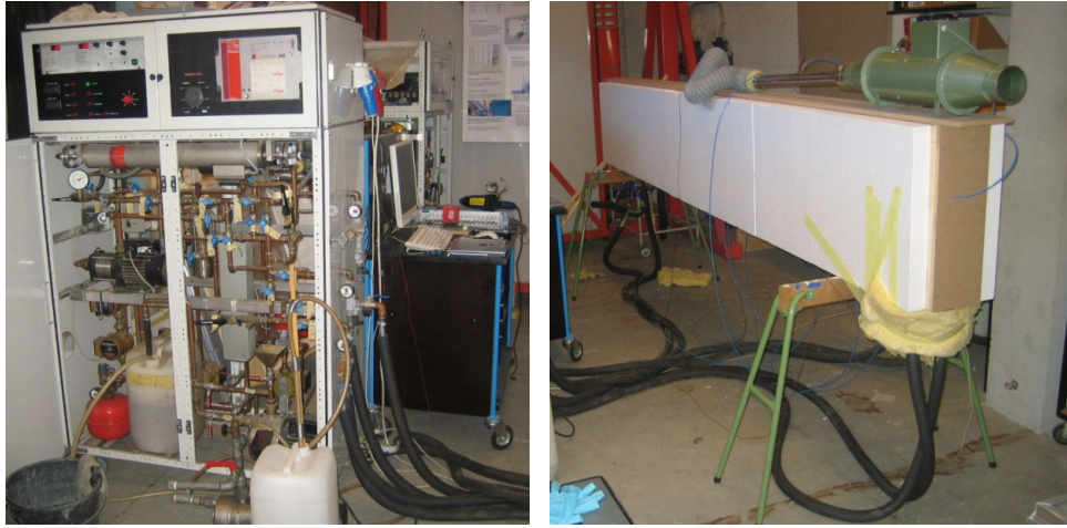
(a) Cooling/heating rack
