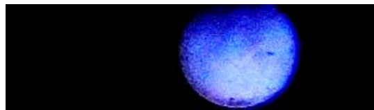
Figure 32 - Combustion quickly proceeds to embrace entire combustion chamber
