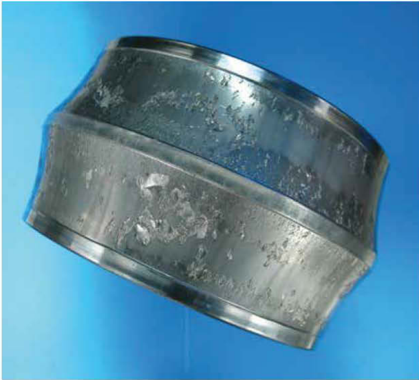
Severely spalled inner-ring of planetary spherical-roller bearing used in wind turbine gearbox
