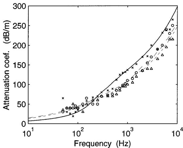
FIG. 5. Attenuation coefficient for glass wool of density  $30 \text{ kg/m}^3$ . The points marked "x" are the measured value for propagation in the X-direction. The points marked "O" are for the Y-direction, and "Δ" is for the Z-direction. The curves were calculated. The full line is for the X-direction, the dashed for Y-direction, and the dotted for Z-direction.
