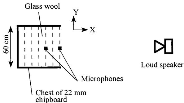
FIG. 1. The measurement setup in the anechoic room. Six slabs of glass wool each with dimension  $10 \times 60 \times 90$  cm were placed in the chest. The distance from chest to loudspeaker was 170 cm.
