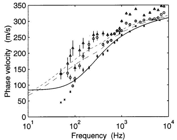
FIG. 4. Phase velocity for glass wool of density 14 kg/m<sup>3</sup>. The points marked “x” are the measured value for propagation in the X-direction. The points marked “o” are for the Y-direction, and “Δ” is for the Z-direction. Measurement uncertainty is shown as vertical error bars. The curves were calculated. The full line is for the X-direction, the dashed for Y-direction, and the dotted for Z-direction.
