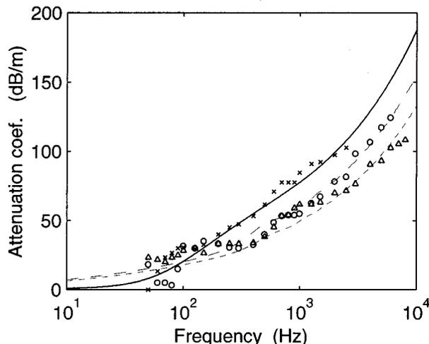
FIG. 2. Attenuation coefficient for glass wool of density  $14 \text{ kg/m}^3$ . The points marked "x" are the measured value for propagation in the X-direction. The points marked "O" are for the Y-direction, and "Δ" is for the Z-direction. The curves were calculated. The full line is for the X-direction, the dashed for Y-direction, and the dotted for Z-direction.
