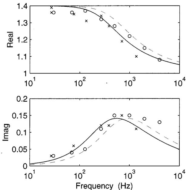
FIG. 3. The complex compressibility of air between fibers. The data are normalized by division with the isentropic compressibility. The “x” points are for density 16 kg/m<sup>3</sup>, and the full line is computed by Eq. (4) with time constant 0.50 ms. The “o” points and the dashed line are for density 40 kg/m<sup>3</sup> with time constant 0.30 ms.
