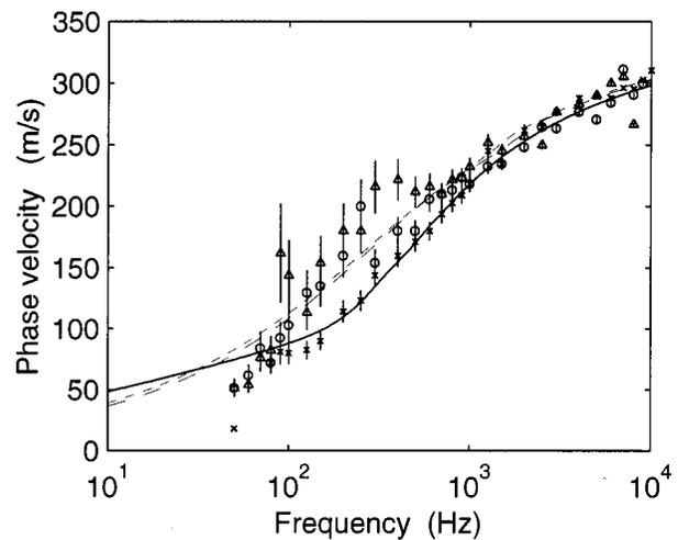
FIG. 6. Phase velocity for glass wool of density  $30 \text{ kg/m}^3$ . The points marked "x" are the measured value for propagation in the X-direction. The points marked "O" are for the Y-direction, and "Δ" is for the Z-direction. Measurement uncertainty is shown as vertical error bars. The curves were calculated. The full line is for the X-direction, the dashed for Y-direction, and the dotted for Z-direction.
