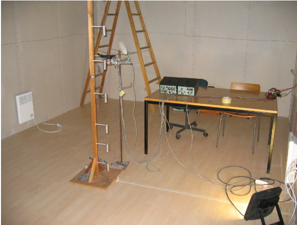
Figure 6.21 Room. Four 500W heating panels (two can be seen here) are installed on each wall. Centrally in the room, measurements of temperatures (air, radiant and operative) are performed as well as air velocity and relative humidity.
