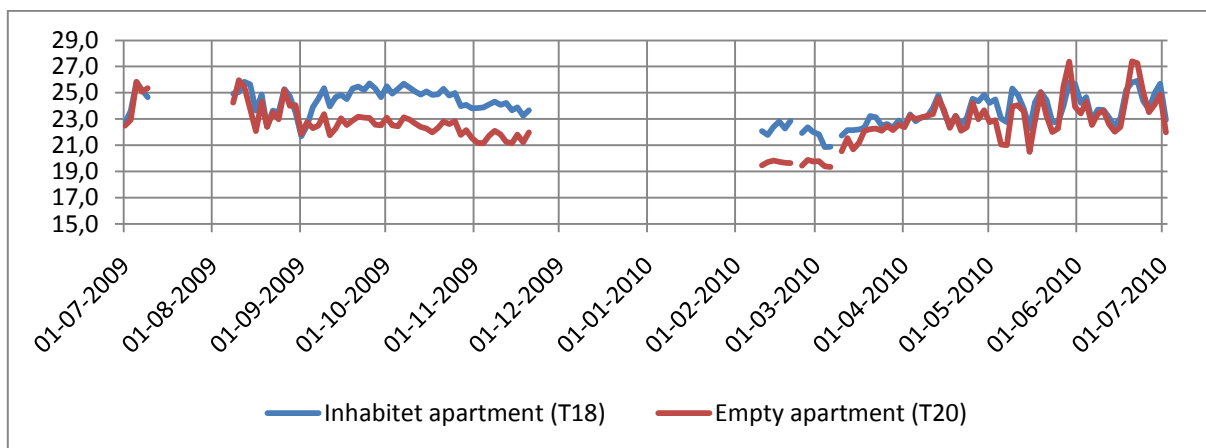
Figure 4 Measured air temperature in kitchens/living rooms from July 2009 to June 2010
