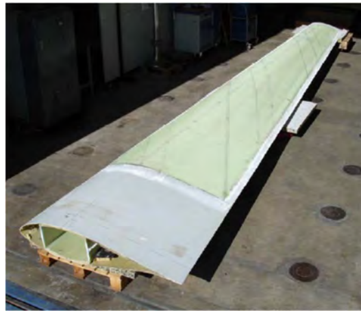
Figure 2.6: Wind turbine blade section after its modification. The extra GFRP UD layers are seen as a light-green layer on top of the blade section with the fiber direction shown by dark lines.
