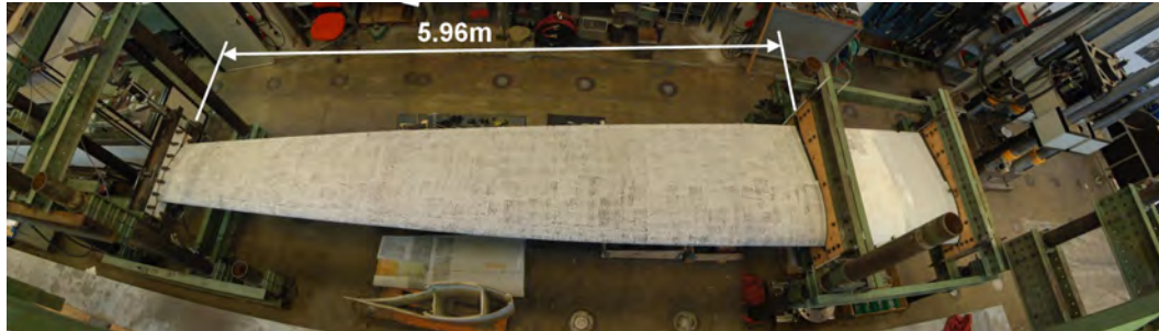
Figure 2.9: Test setup for blade section in test hall.
