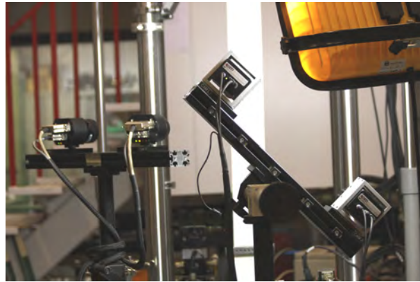
Figure 4.22: Photo of DIC systems setup. Left – small-scale DIC system; Right – full-scale DIC system. A composite beam appears white.
