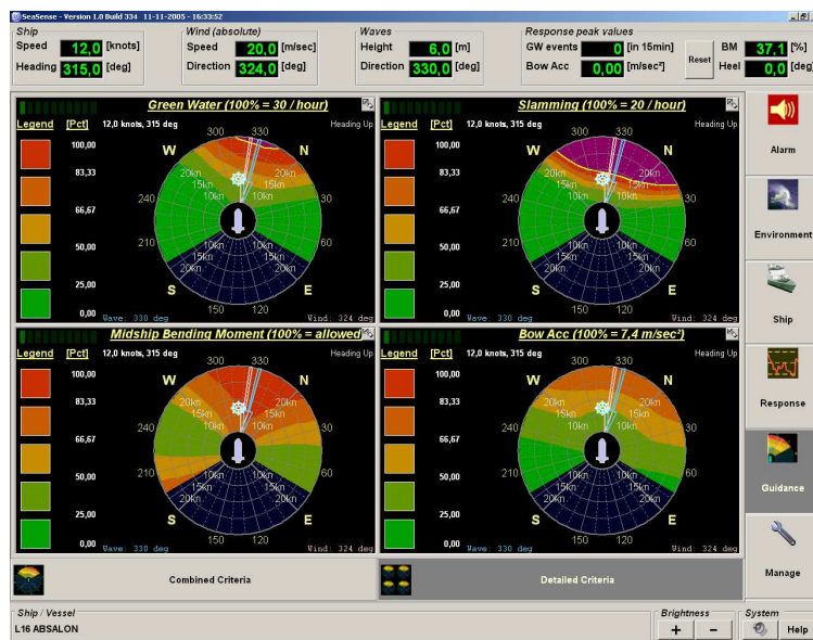
FIGURE 2. Examples of guidance plots from the SeaSense system. Nielsen et al. [34]
