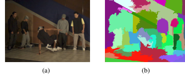
Fig. 3. Segmented color image for the first frame of the sequence breakdancers ( QP = 28 ). a) Reconstructed color image; b) Segmentation
