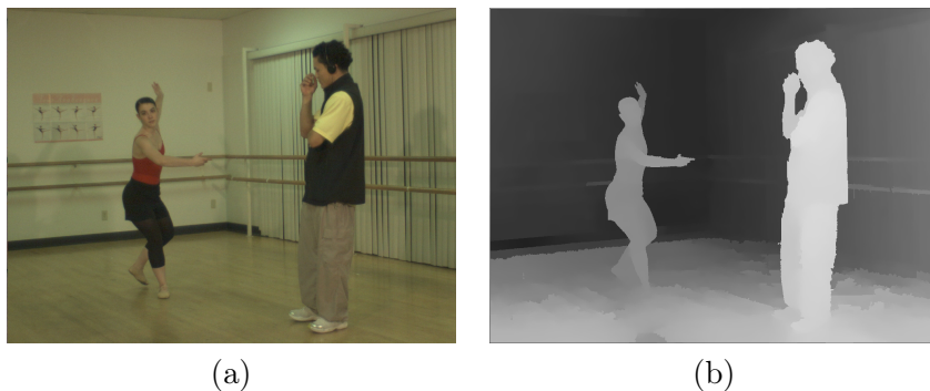
Figure 1.1: A color image (a) and the corresponding depth map (b) from the Ballet dataset [17]. The brighter the pixels, the closer the object. Frames of other test sequences are reported in App. B.
