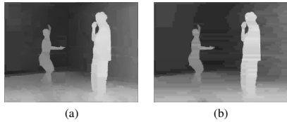
Fig. 8. Visual comparison of the compressed depth maps at 0.025 bpp (ballet sequence) (a) proposed scheme; (b) H.264/AVC.
