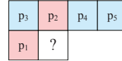
Fig. 2: Template selection: pixels p_1 and p_2 are fixed; one additional pixel among p_3 , p_4 , and p_5 can be included in the template. “?” indicates the current pixel being encoded.
