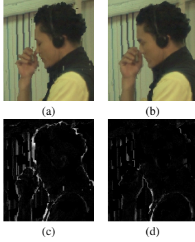
Fig. 5: Visual quality comparison versus total depth bit rate: detail of the synthesized view from uncompressed texture, Ballet sequence, frame 0. H.264/AVC Intra, 34.73 dB @ 726 kbit/s (a), Proposed, 37.67 dB @ 723 kbit/s (b), absolute errors on the luminance components (with same scale) between synthesized views obtained with uncompressed depth data and H.264/AVC Intra (c) and Proposed (d).
