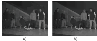
Figure 7: Visual comparison (breakdancers 8-view dataset, view 4 at 0.01 bpp) : a) H.264 encoding and b) proposed method
