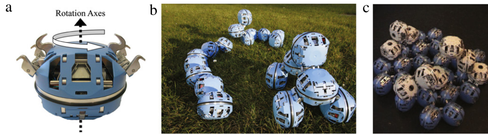
Fig. 3. (a) A single ATRON module: on the top hemisphere the two male connectors are extended, on the bottom hemisphere they are contracted. (b) Different configurations of ATRON modules. (c) Meta-modules for self-reconfiguration.
