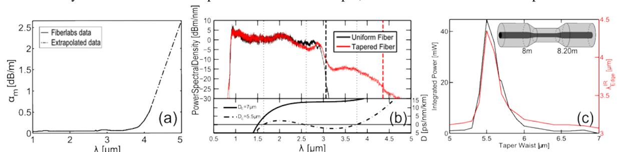
**Fig. 1** (a) ZBLAN material loss (solid) provided by Fiberlabs Inc., Japan. (b) Top: SC spectrum in a 10 m uniform (black) and tapered (red) fiber with the -30 dB IR edge indicated by a dashed line. Below: Dispersion (D) of the uniform fiber ( $D_c=7\ \mu\text{m}$ ) and the taper waist ( $D_c=5.5\ \mu\text{m}$ ). Dotted lines are ZDWs at taper waist. (c) Integrated power above 3.06  $\mu\text{m}$  versus taper waist core diameter for a 20 cm long symmetric taper with start at 8 m (see inset).
