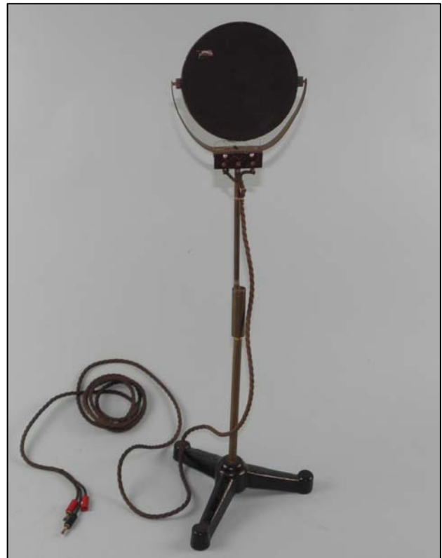
Instrument for measuring radiation, constructed by Bisgaard.
