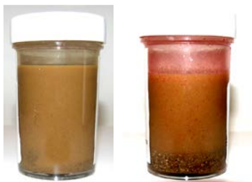
Figur 1: Hydrofob farvetest (OilScreenSoil (Sudan(IV))®) – venstre: negativ, højre: positiv for DNAPL
