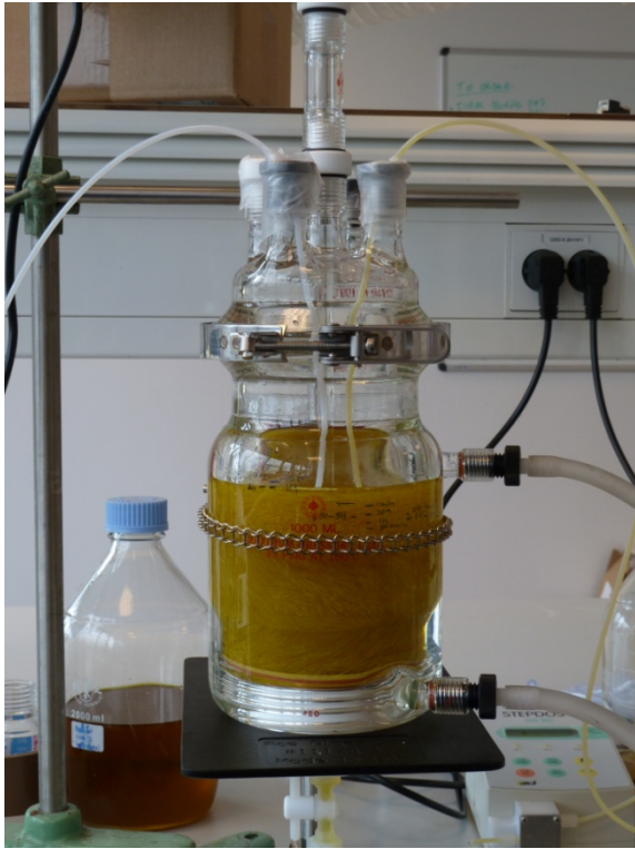
Continuous stirred tank reactor for enzymatic biodiesel production
