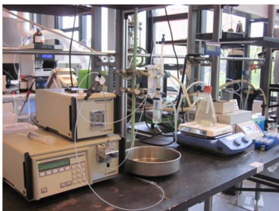
Packed bed reactor for transamination
