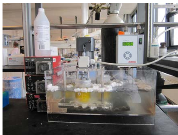
Stirred tank reactor for enzymatic biodiesel production
