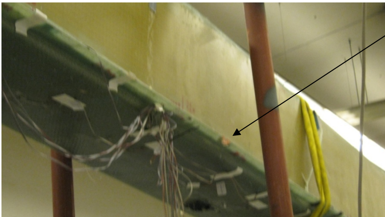
Figure 83 Steel pipe supporting the blade. There is a damage in the connection between the web and the cap
