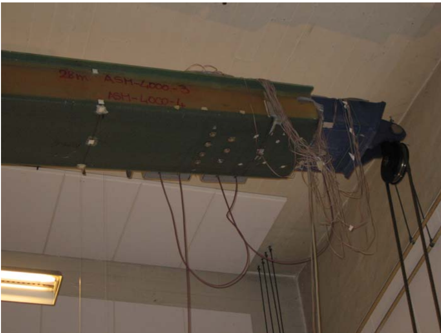
Figure 58: The loads was tranfered to the boxgirder with at steelinsert in the tip. The steel insert reaches 700 mm inside the girder and is fastened to the girder with adhesives and bolts.
