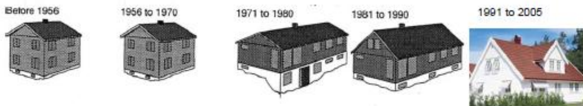
Figure 11. Stereotypes of single-family houses, dependent on the year of construction [1]
