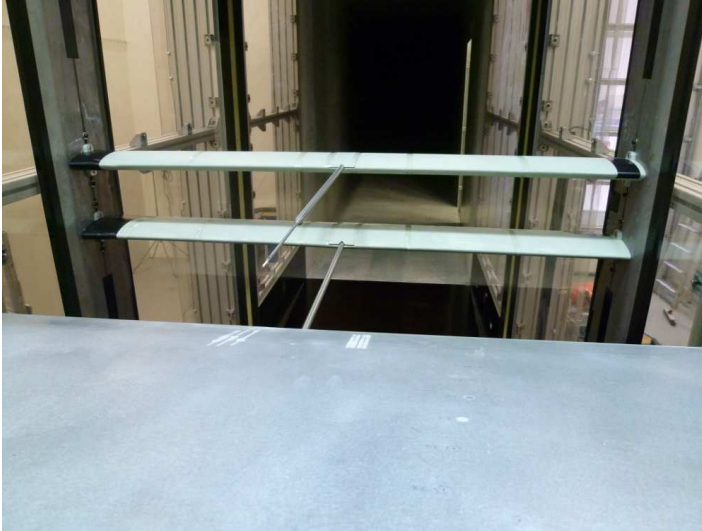
Figure 2. Slanted hot-wire holders set-up
