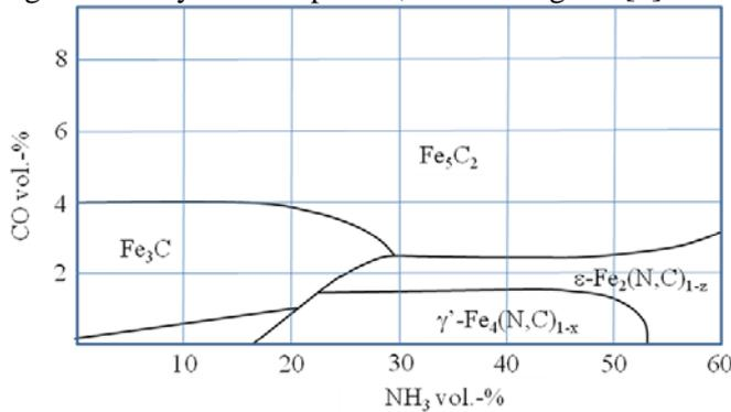
Fig. 3: Phase stability of Fe-N-C phases at 500 °C in NH<sub>3</sub>-CO-H<sub>2</sub> gas mixtures [10].
