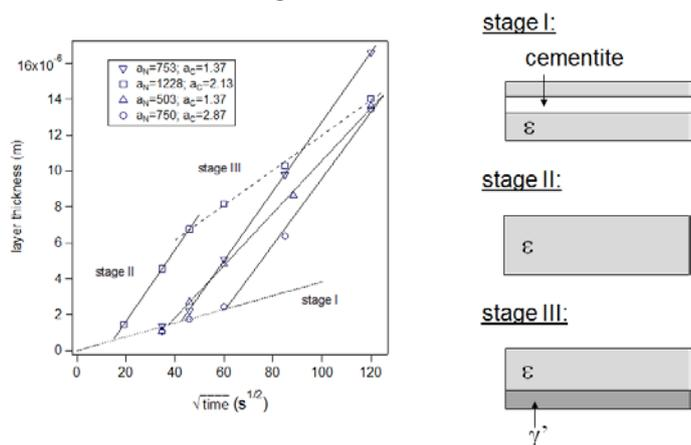
Fig.10: Kinetics of compound layer growth during nitrocarburizing of iron can be subdivided in 3 stages (I,II,III). Data points are for various combinations of nitrogen activity ( $a_N$ ) and carbon activity ( $a_C$ ) in the gas phase [5,13].
