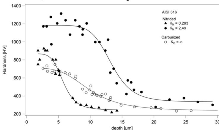
Fig.16: Hardness-depth profiles of AISI 316 nitrided at 445 °C (718 K) for 22 h in NH<sub>3</sub>-H<sub>2</sub>-N<sub>2</sub> gas mixtures, with nitriding potentials indicated, or carburized at 507 °C (780 K) for 6 h in a CO-H<sub>2</sub>-N<sub>2</sub> gas mixture. The lines are fitted by a Hill equation and show a sharper case-core transition for nitrided than for carburized material [42].
