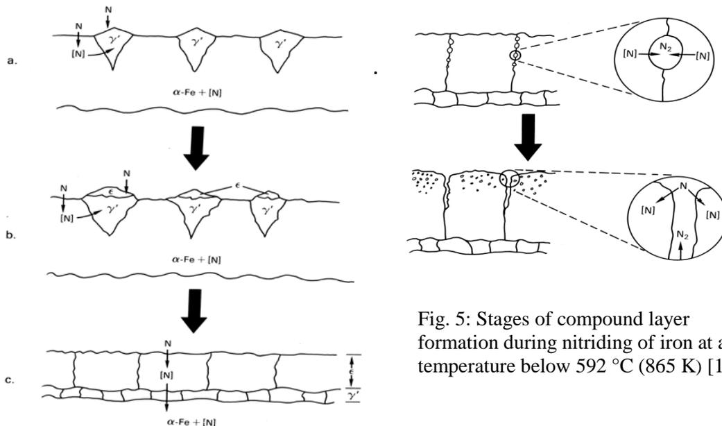
Fig. 5: Stages of compound layer formation during nitriding of iron at a temperature below 592 °C (865 K) [12].
