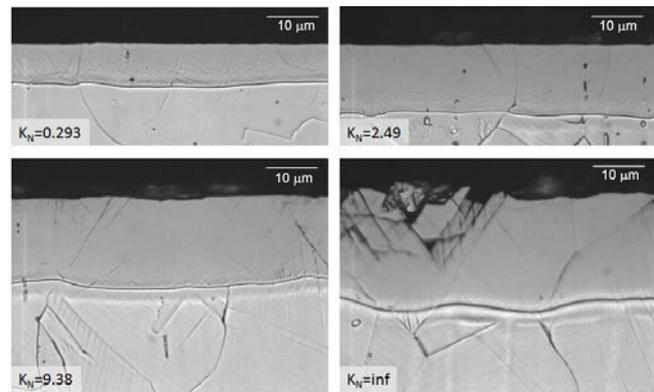
Fig.15: Cross sections of AISI 316 nitrided at 445 °C (718 K) for 22 h in NH<sub>3</sub>-H<sub>2</sub>-N<sub>2</sub> gas mixtures, at various nitriding potentials,  $K_N$  [41,46] .
