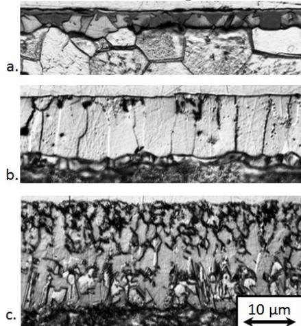
Fig.9: Compound layers obtained after nitrocarburizing at T=570 °C (843 K) for t=3 h.
