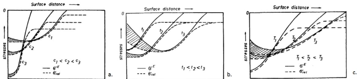
Fig. 13: Evolution of residual stress profiles in the diffusion zone with concentration of nitride formers,  $c$  (a), with nitriding time  $t$  (b), with nitriding temperature,  $T$  (c). The shaded areas mark stress relaxation as a consequence of decarburization and overaging ( $\sigma_{rel}$ =relaxation stress;  $\sigma_E$ =elastic stress due to volume mismatch) [37].
