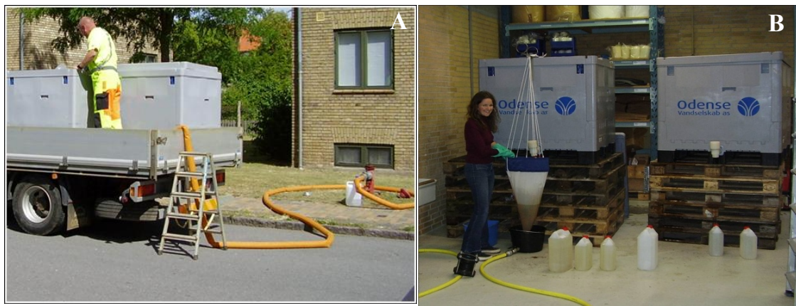
Figure 2-1. A) Sampling from a fire hydrant into containers with single use plastic bags. B) filtration of the samples through a series of nets. Photos: S.C.B. Christensen and E. Nissen
