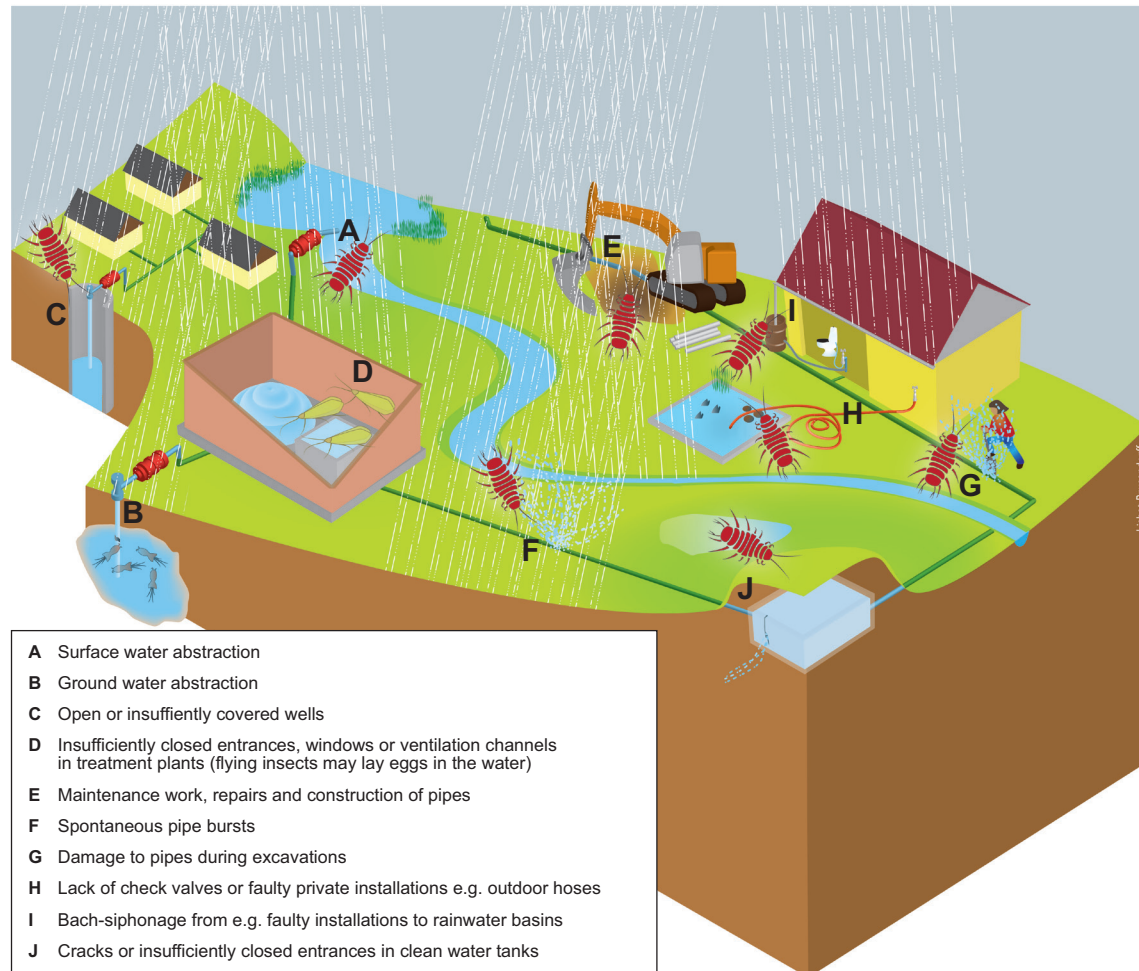
Figure 3-2. Potential entry points of invertebrate intrusion into drinking water systems. A. aquaticus represents ingress of surface water invertebrates, while the invertebrates at B come from the groundwater and D by air. Graphical design: L. Brusendorff.
