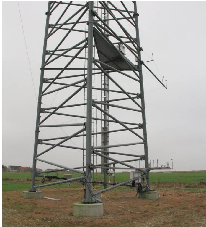
Figure 7 The Avent 3B nacelle lidar mounted on a platform 10 m above the ground at the DTU test site.
