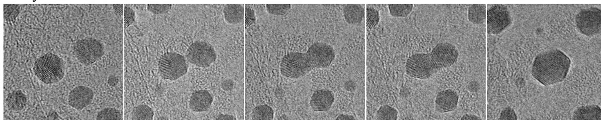
ETEM image sequence of Au/graphene in 200 Pa H<sub>2</sub> at 104°C. The image series shows different stages of two Au particles coalescing resulting in a single Au particle. Image dimensions: 18x18 nm.
