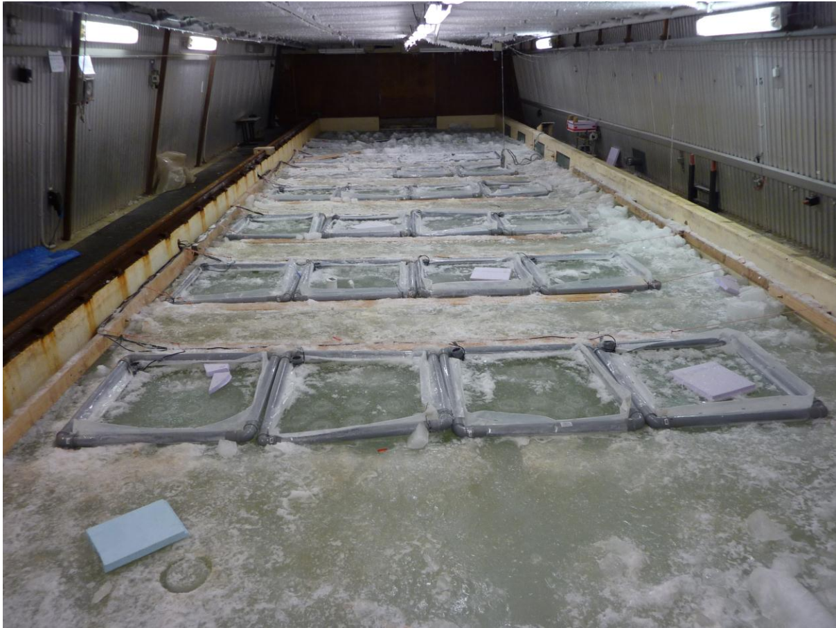
Fig. 1: The experimental mesocosms floating in an environmentally controlled ice tank of the Hamburg Ship Model Basin. The foam pads on some of the mesocosms mark the compromised ones after they have been sampled. Note that the lights were on only during sampling (at maximum 2 hours per day) and the rest of the time, the tanks were in darkness.
