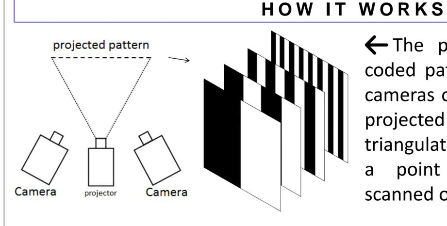
The projector projects a binary coded pattern on to the object. The cameras captures the result for every projected pattern, and by using triangulation, its possible to construct point cloud representing the scanned object.
