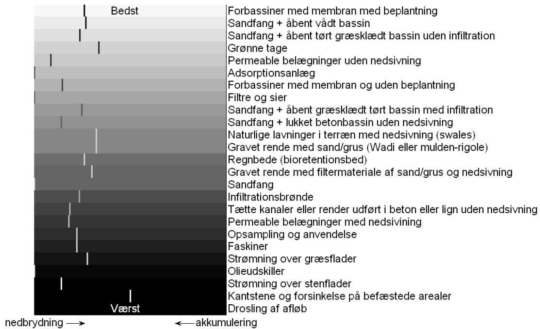
Figure 5 – Ranking of BMPs for the removal of metals (Cd, Cr, Cu, Ni, Pb).
