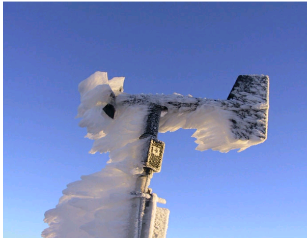
Figure 7.10: Vane covered by ice (source EUMETNET [20])
