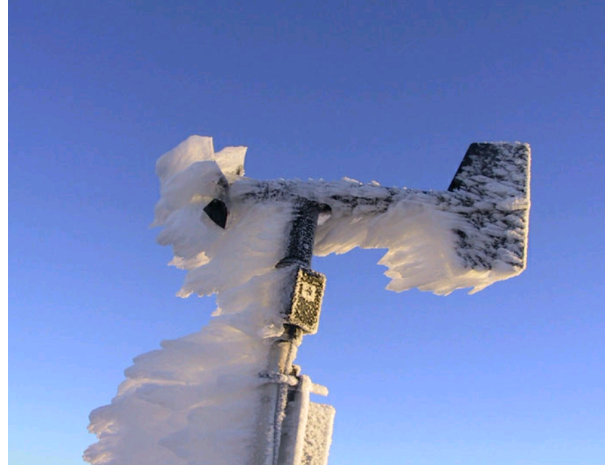
Figure 7.10: Vane covered by ice (source EUMETNET [20])
