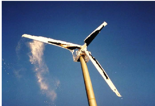
Figure 8.6: Black coated blade with ice shedding[35]
