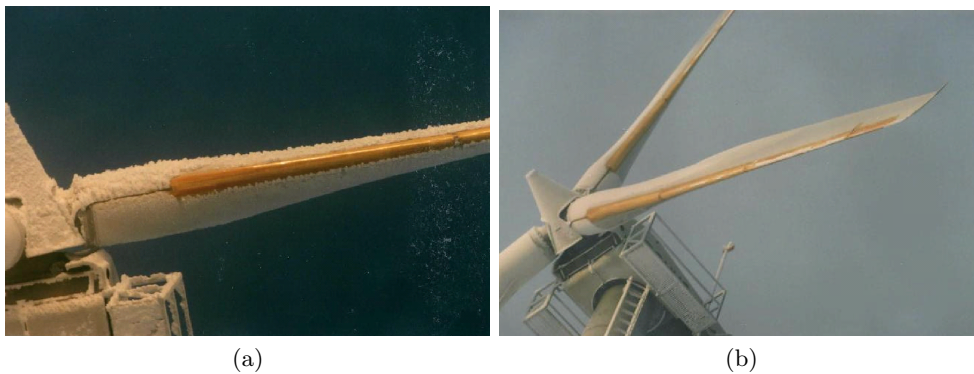
Figure 8.2: Leading edge electrical heating of a blade - Pictures[35]. (a) Severe icing - (b) Slight icing
