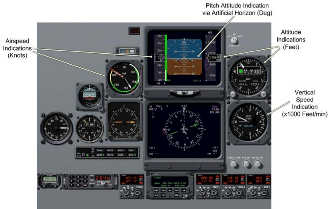
Figure 5: Typical instrument panel showing ASI, AI, VSI, ALT and DG instruments
