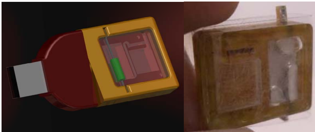
Fig.3. Micro coffee machine: conceptual design and final product held between two fingers.
