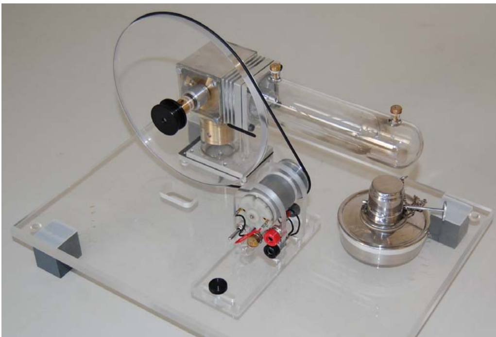
Figure 3. Transparent Stirling engine used for second assignment
