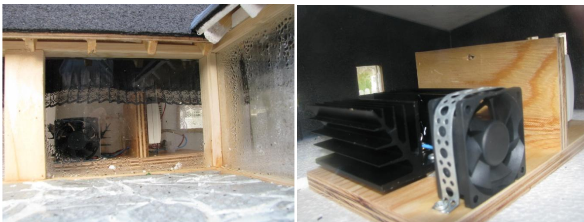
Figure 5. In the implementing face, the students have mounted a heating unit, an adjustable thermostatic switch, and a small fan to circulate air.
