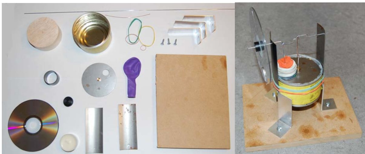
Figure 1. Stirling engine built by students on first day of the course.
