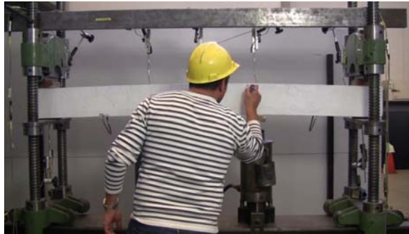
Figure 1. Test set-up for the concrete beam with student marking the cracks (traditional)
