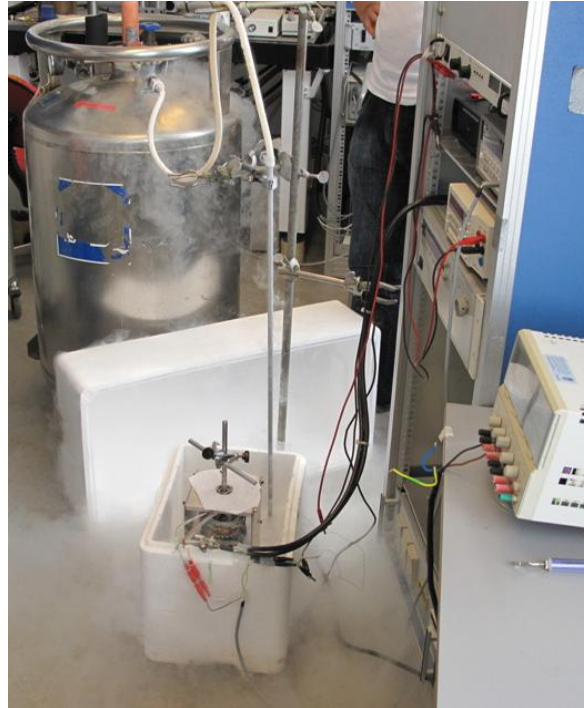
Figure 5. The HTS machine prototype setup after cool-down and during testing.
