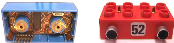
Figure 1. Left: the internals of a building block with micro processor and communication channels. Right: example of input (sensor) building block that contains two microphones.
